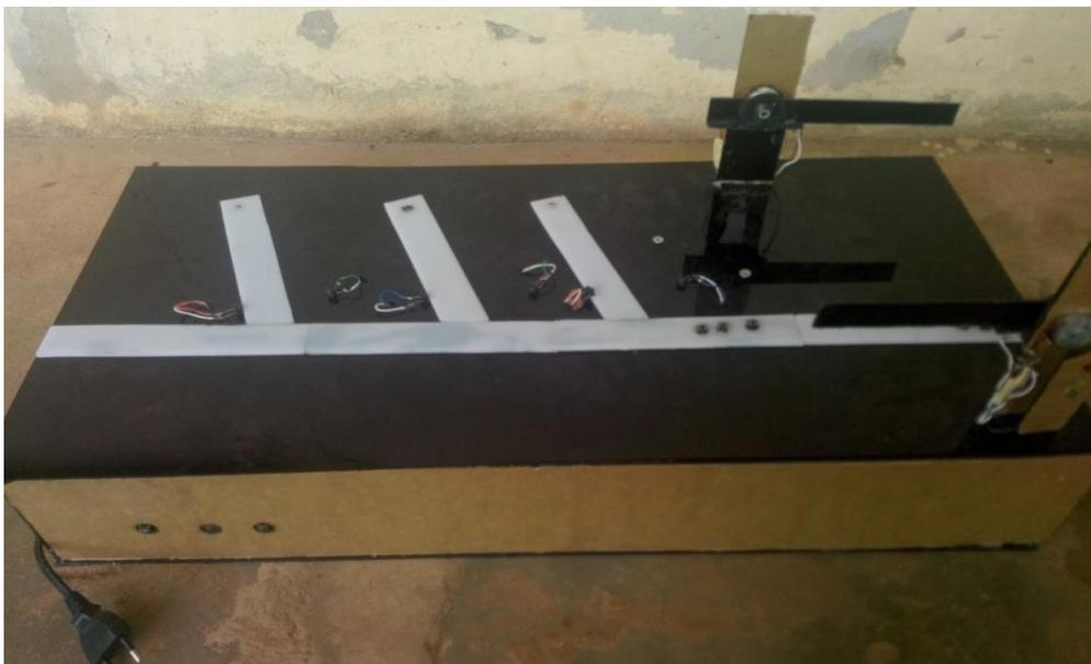
Figure 12: Picture of Prototype of the Computerized Railway Station Traffic Control System
