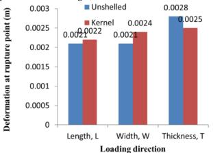
Figure 6. Deformation at rupture point of unshelled and kernel of Dialium guineense fruit across different loading directions.
