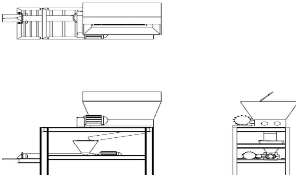
Figure 2: Orthographic view of the plastic recycling machine
