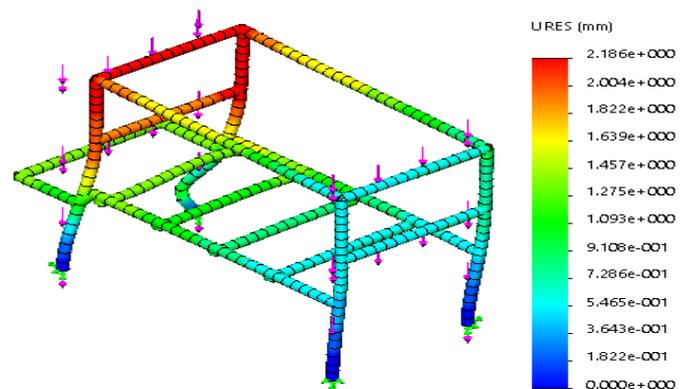
Figure 6 Resultant displacement of the machine frame during buckling test
