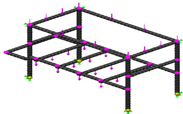
Figure 3 Frame solid mesh model with normally acting uniformly distributed load
