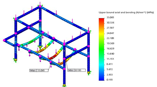
Figure 4: FE analysis of the stress distribution within the machine frame members
