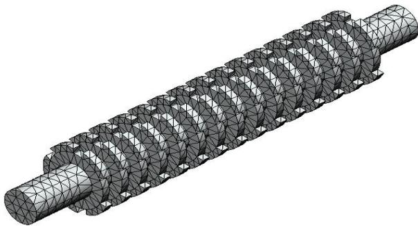
Figure 8: Solid mesh model of the shredder shaft
