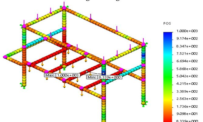
Figure 7: Factor of safety distribution on the machine frame members
