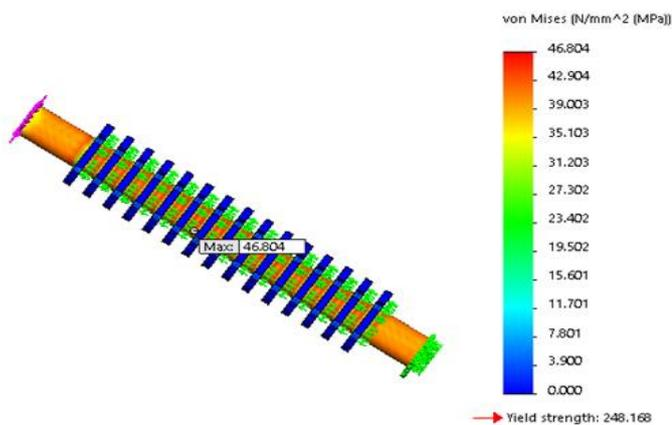
Figure 9: FE model of the stress distribution in the shredder shaft due to torsion
