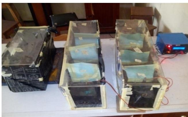
Figure 1. Electro bioremediation experimental set up
