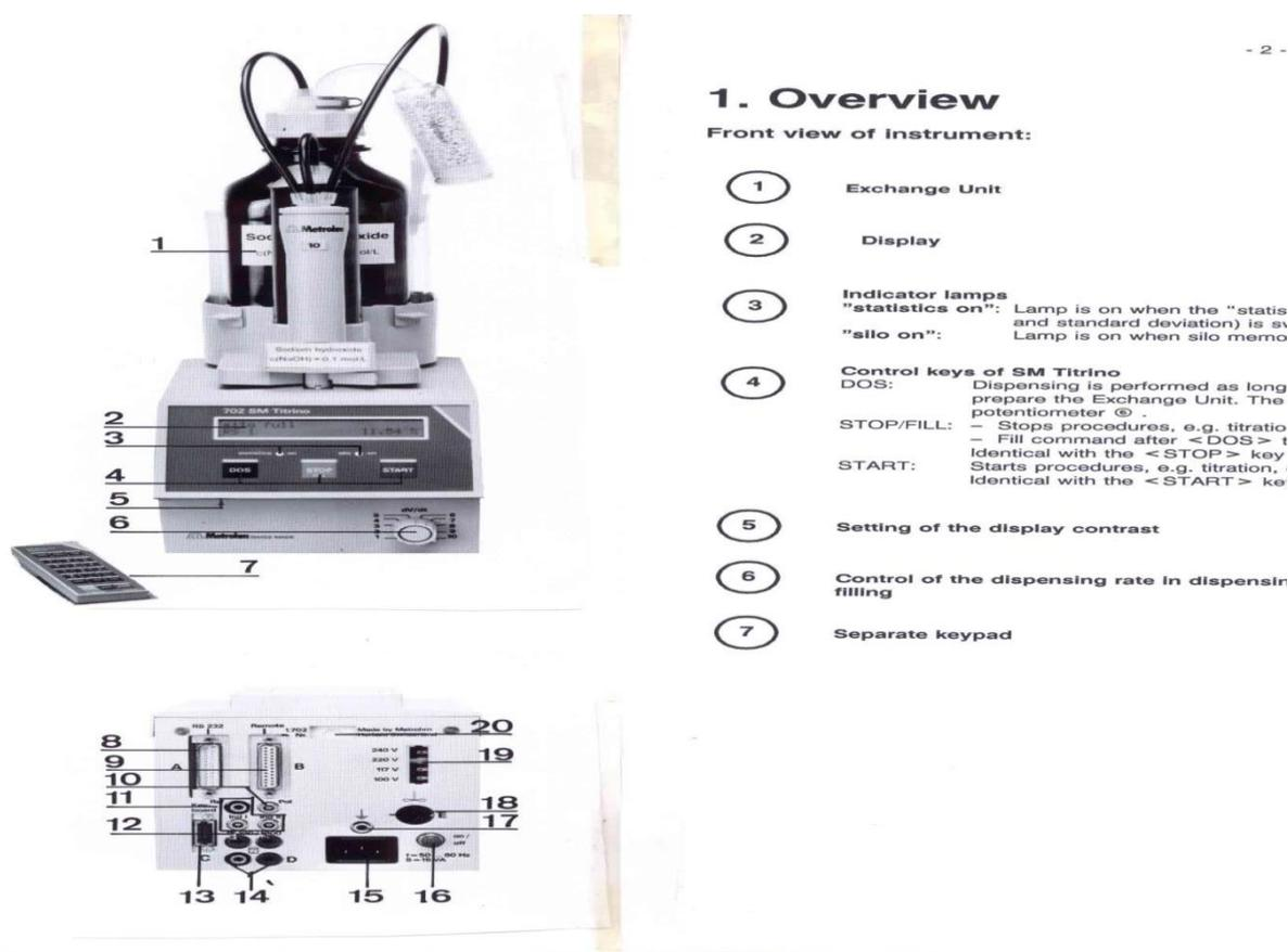
Figure 1: Volumetric titration system (Source: [www.astm.org/standards](http://www.astm.org/standards))
