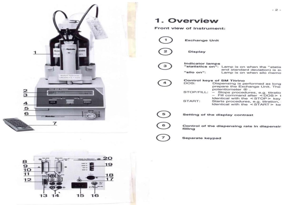
Figure 1: Volumetric titration system (Source: [www.astm.org/standards](http://www.astm.org/standards))
