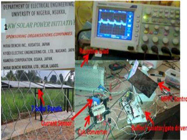
Figure 10 Laboratory Setup
