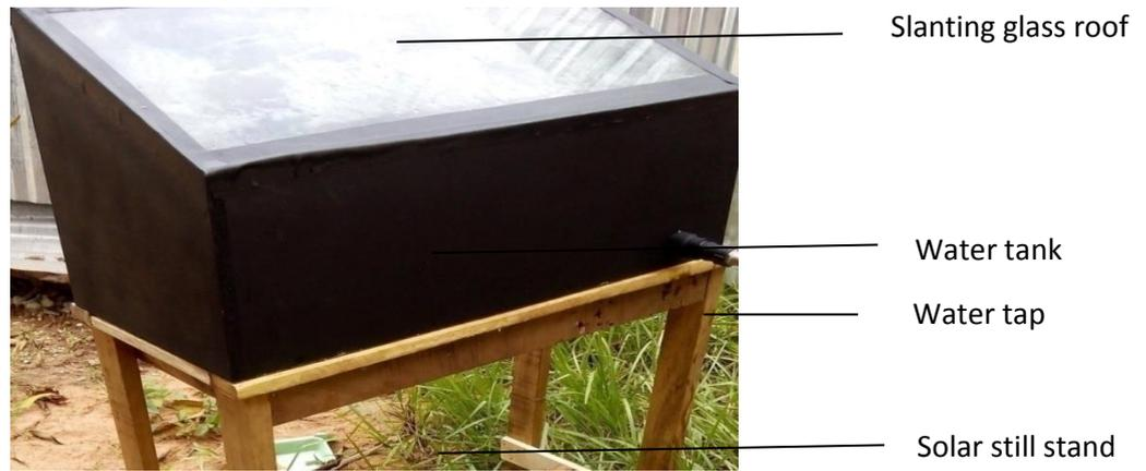
Figure 2: Isometric view of the slanting-type solar water distillation (SSWD) kit
