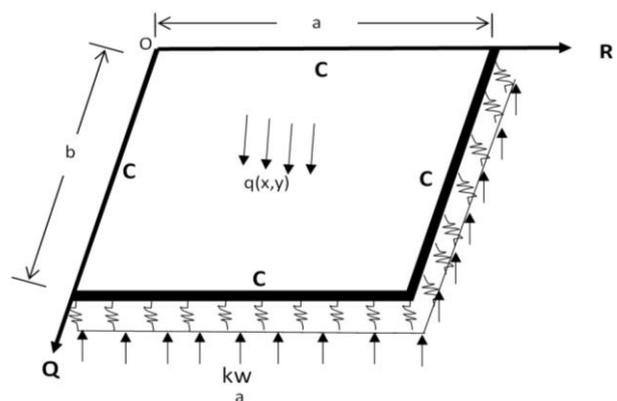
Figure 1: An all clamped rectangular thin plate on elastic foundation
