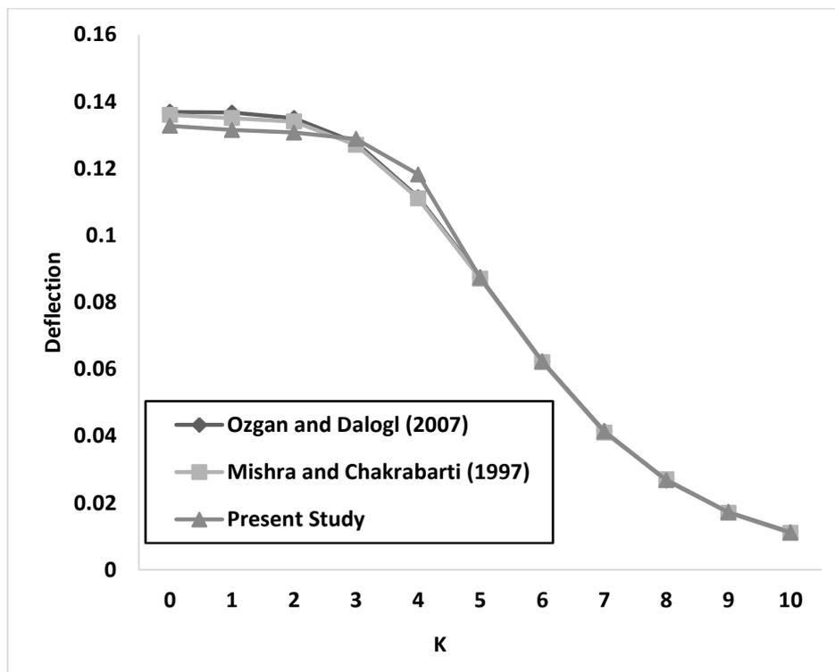
Fig. 2 Variation of the non dimensional central deflection with K for clamped supported plate subject to concentrated load
