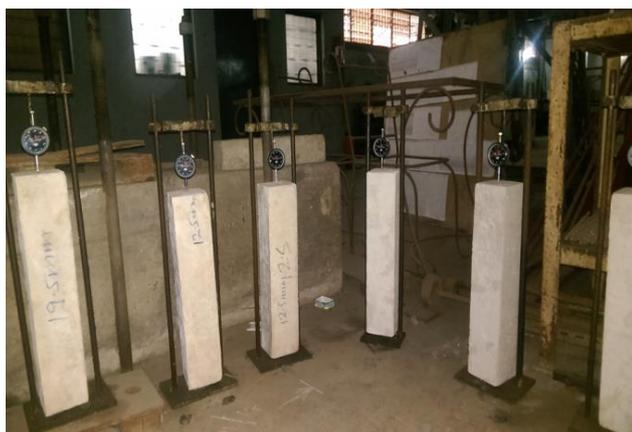
Plate 1: Laboratory setup for measuring shrinkage strain in the specimens
