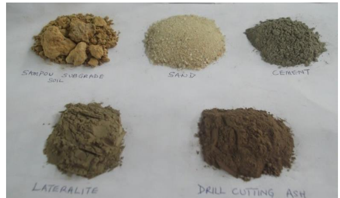
Figure 2: Soil sample, additives and binder used
