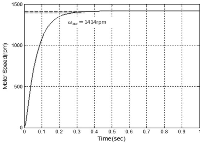
Figure 6: Speed Response of DC Motor for running an Emergency Lube Oil Pump in H25 Hitachi Gas Turbine Generator
