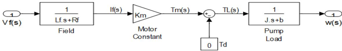
Figure 3: Block Diagram of Field-Controlled DC Motor for Driving Lube Oil Pump
