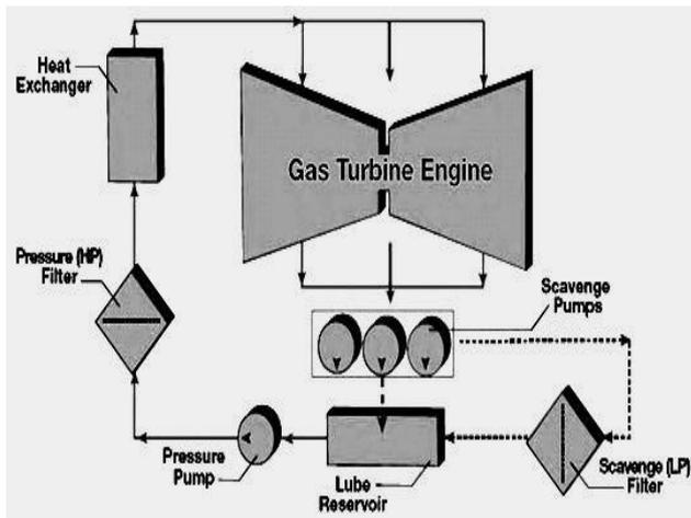
Figure 1: Simplified Diagram of the Gas Turbine Lubrication System, Source:[11]
