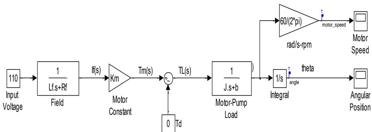
Figure 5: Simulink Model of Lube Oil Pump Field-Controlled DC Motor
