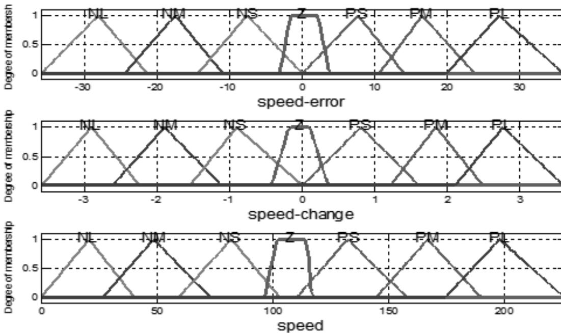
Figure 11: Adjusted Triangular and Trapezoidal inputs and Output Membership Functions.
