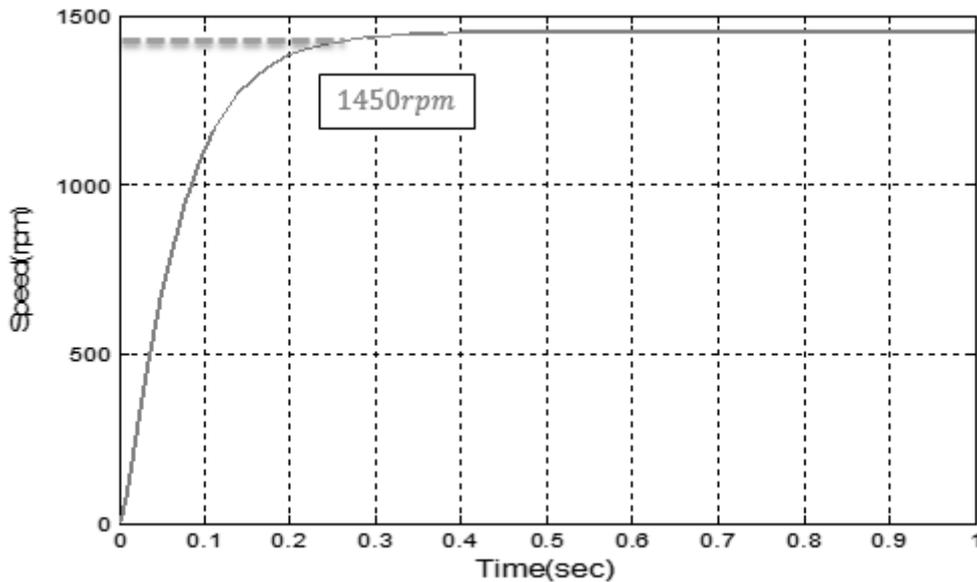
Figure 12: Speed Response of DC Motor with Adjusted FLC for Running an Emergency Lube Oil Pump in H25 Hitachi Gas Turbine Generator
