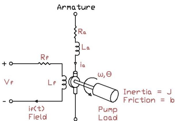
Figure 2: DC Motor wiring diagram [5].
