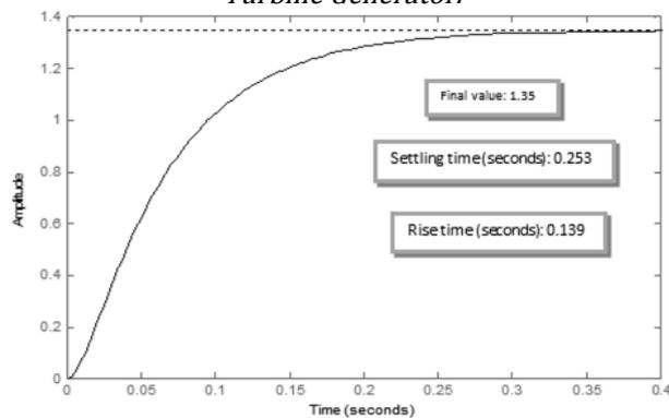
Figure 8: Response of DC Motor for running an Emergency Lube Oil Pump in H25 Hitachi Gas Turbine Generator
