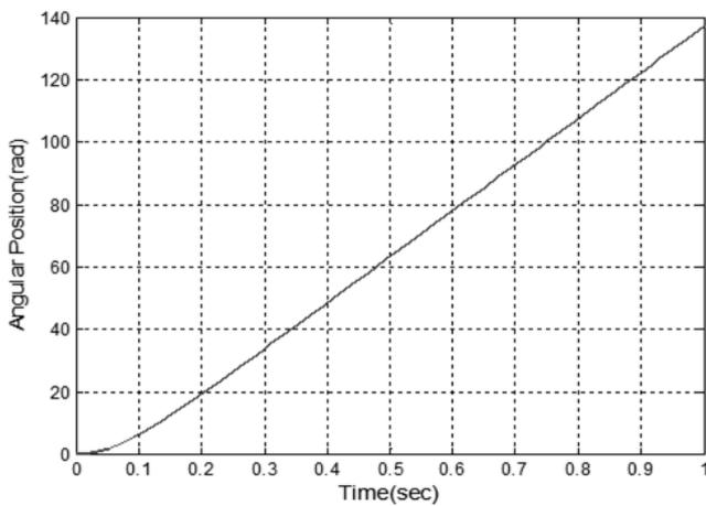
Figure 7: Angular Position Response of DC Motor for running an Emergency Lube Oil Pump in H25 Hitachi Gas Turbine Generator.
