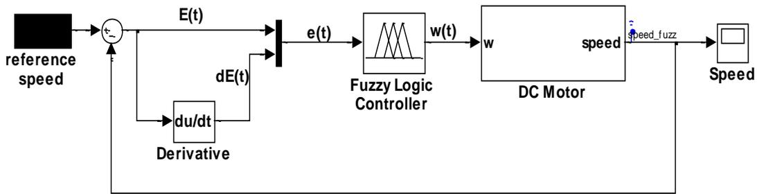
Figure 9: Simulink Model of FLC and DC Motor.
