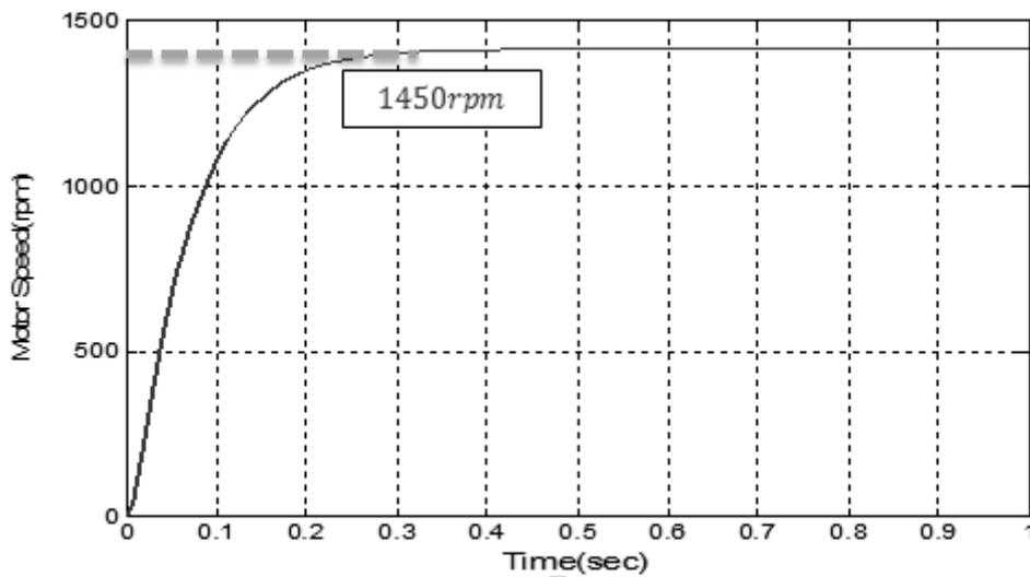
Figure 10: Speed Response of DC Motor with FLC for Running an Emergency Lube Oil Pump in H25 Hitachi Gas Turbine Generator
