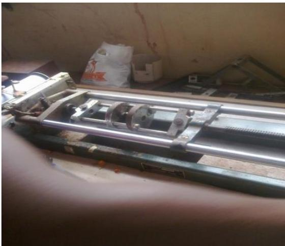
Figure 3: Monsanto tensiometer for compression tests
