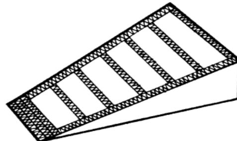
*Fig. 9: Stinger bead hardfacing pattern for smaller aggregates [53]*
