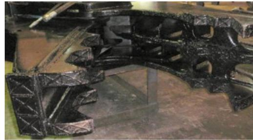
*Fig. 7: Waffle hardfacing pattern [56]*
