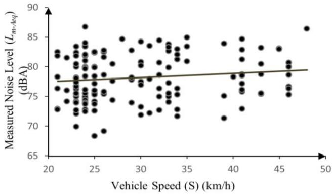
Figure 3: Variation of Noise Level with Vehicle Speed
