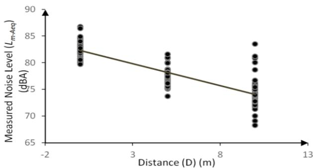
Figure 5: Variation in Noise level with Distance
