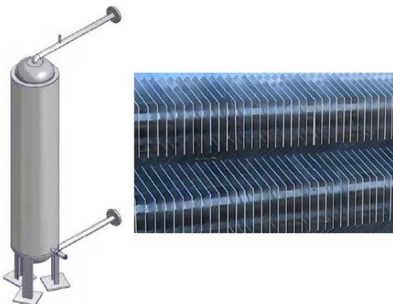
Figure 3: Test storage module using NaNO<sub>3</sub> PCM showing the full module and the fins [35]
