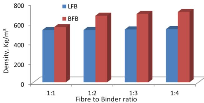
Figure 1: Comparison of Densities of LFB and BFB at different compositions
