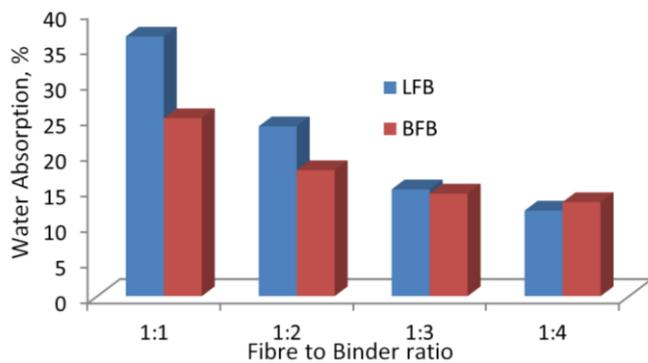
Figure 2: Percentage water absorption of LFB and BFB at different compositions
