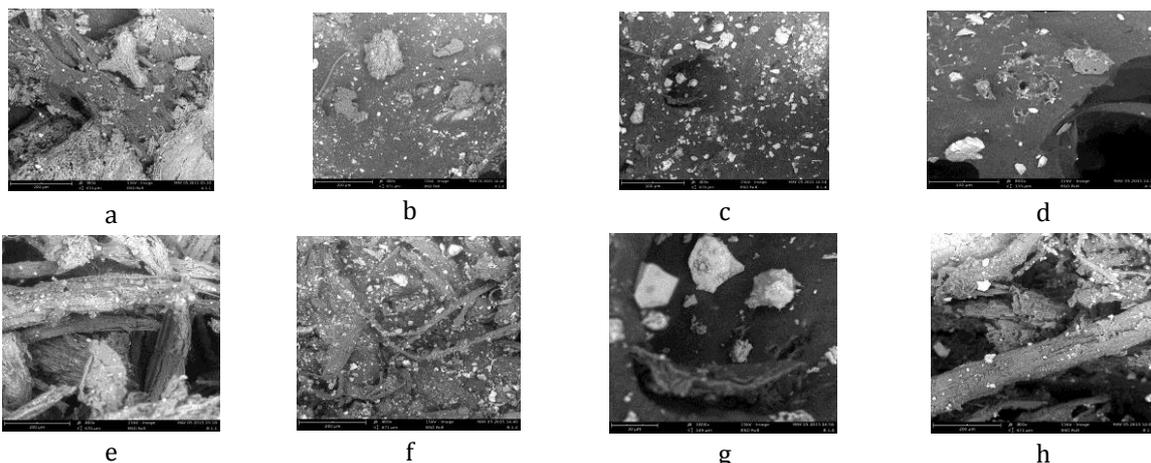
Plate 1: SEM Micrograph of the *Piliostigma thonningii* L. fibre boards (400X)
