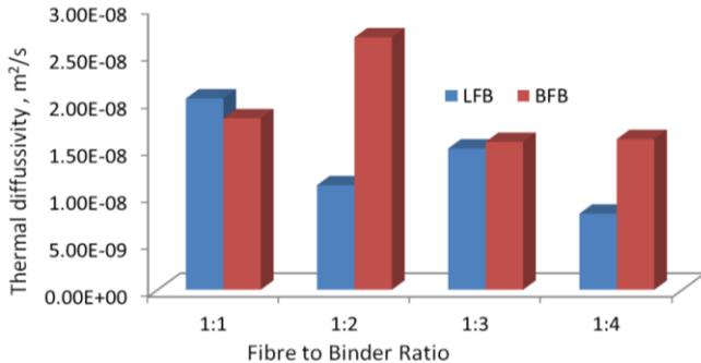
Figure 5: Thermal diffusivity values for LFB and BFB at different composition
