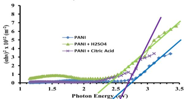
Figure 2. Plot of  $(\alpha h\nu)^2$  versus Photon Energy (eV) for pure PANI, PANI +  $H_2SO_4$  and PANI + Citric acid
