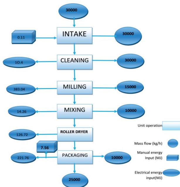
Fig 3: Energy and material balance diagram of breakfast cereal production operations.
