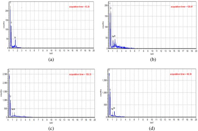
*Figure 10: EDS of C. populnea fibers with (a) untreated (b) treated with NaOH (c) treated with AC (d) treated with EDTA*
