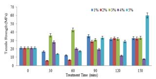
*Figure 5: Tensile strength of EDTA treated C. populnea fibers*
