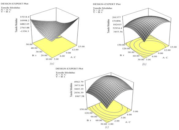
*Figure 8: 3-D response surface of tensile modulus of treated C. populnea fibers with (a) NaOH (b) AC (c) EDTA*
