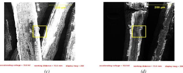
Figure 9: SEM of C. populnea fibers: (a) untreated (b) treated with NaOH (c) treated with AC (d) treated with EDTA
