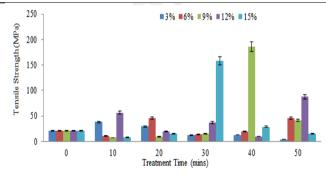
Figure 1: Tensile strength of NaOH treated C. populnea fibers
