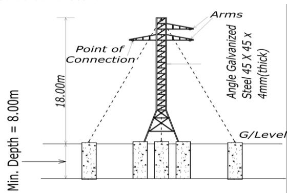
Figure 2: Front view of dead end tower
