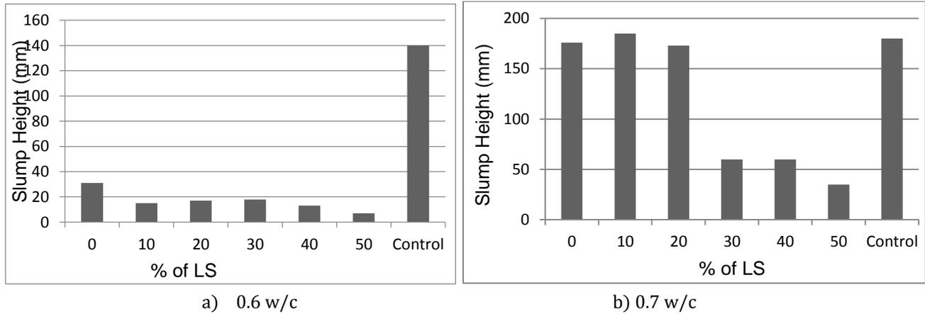
Figure 1: Effect of Replacement on Workability (1:1.5:3 mix)
