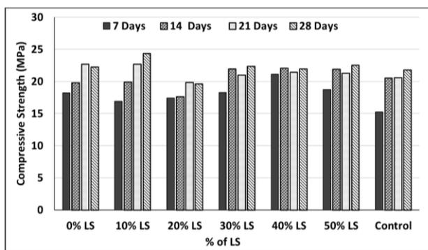
Figure 2: Variation of Compressive Strength with Age at Different % of LS (1:1.5:3 mix and 0.6 w/c)
