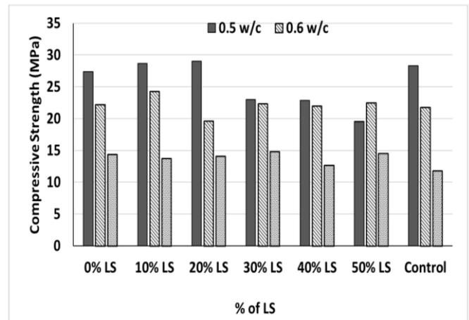
Figure 4: Variation of 28<sup>th</sup> Day Compressive Strength with Water/Cement Ratio at Different % of LS (1:1.5:3 mix)
