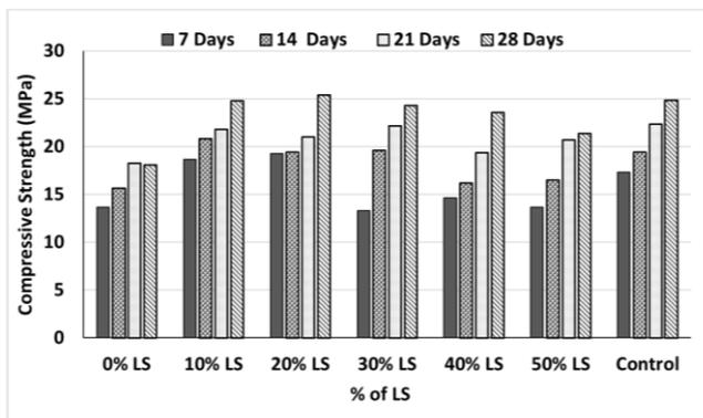
Figure 3: Variation of Compressive Strength with Age at Different % of LS (1:2:4 mix and 0.6 w/c)
