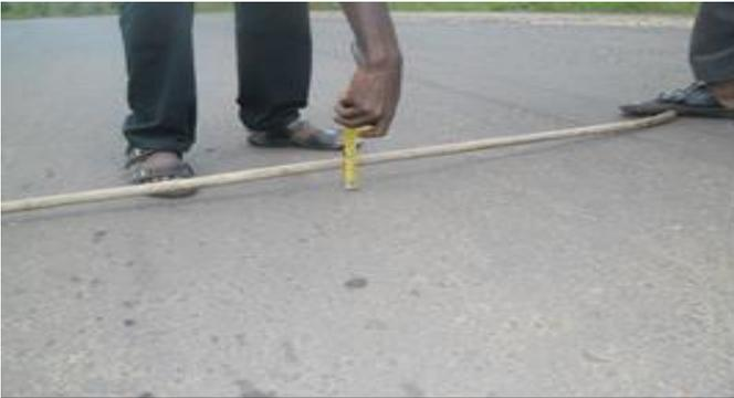
Plate 1: Depressed Portion of Carriageway (Chainage 2+750 - 2+850)
