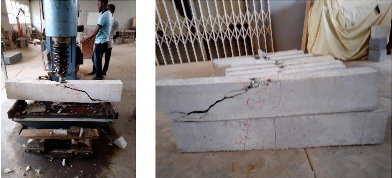
Figure 7: Beam Test Set Up and Tested Beams
