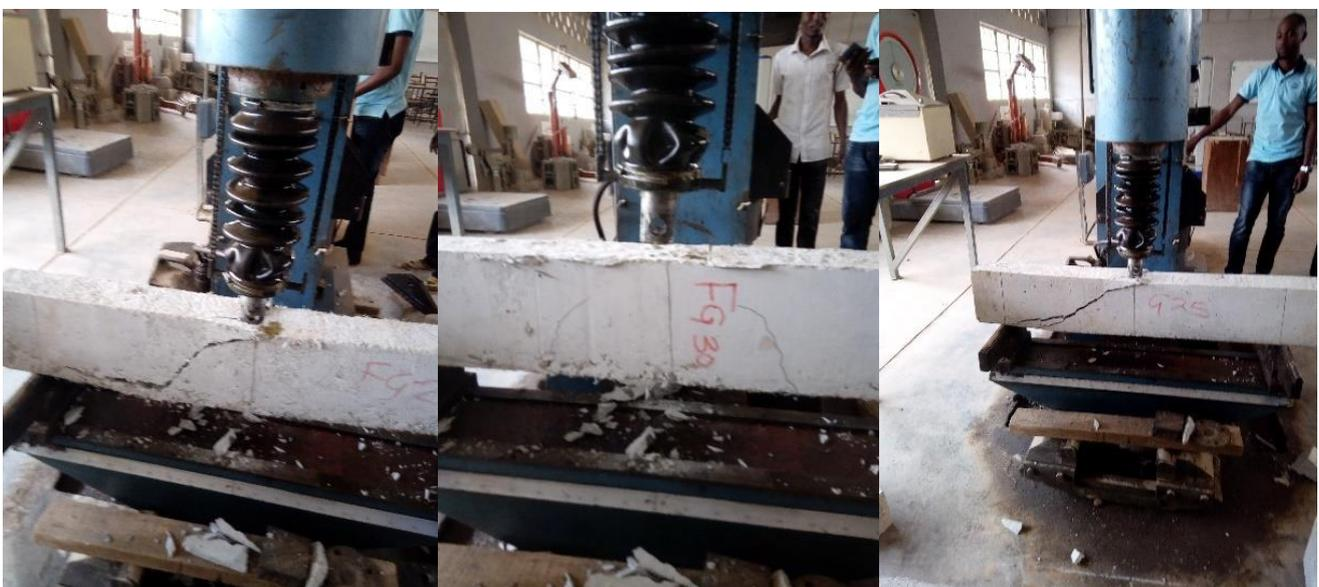
Figure 8: Shear Failures in Beam Test
