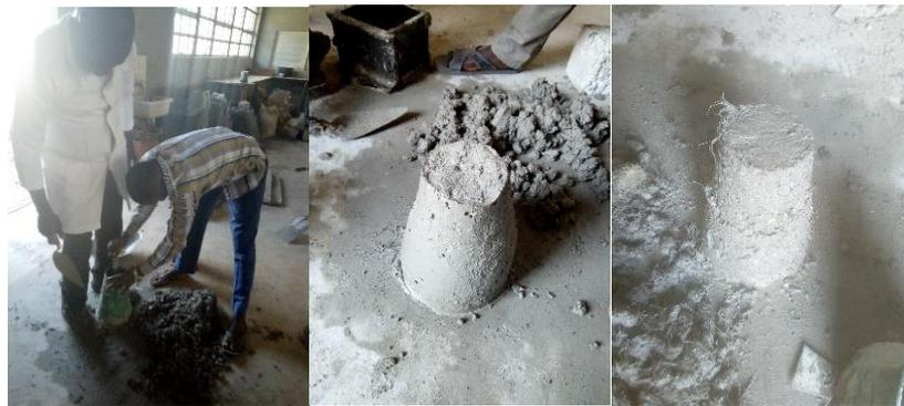
Figure 5: Slump Test to Determine Mix Workability
