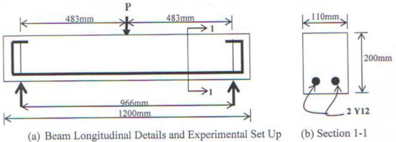
Fig 4: Beam Details and Test Setup
