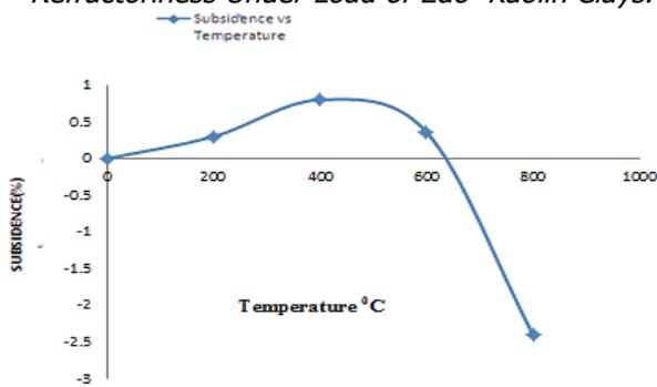
Fig. 7: The Subsidence - Temperature curve of the Refractoriness Under Load of Kebbi Kaolin Clays.
