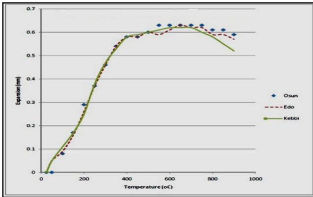
Fig. 1 Thermal Expansion Curves of the Clay Samples
