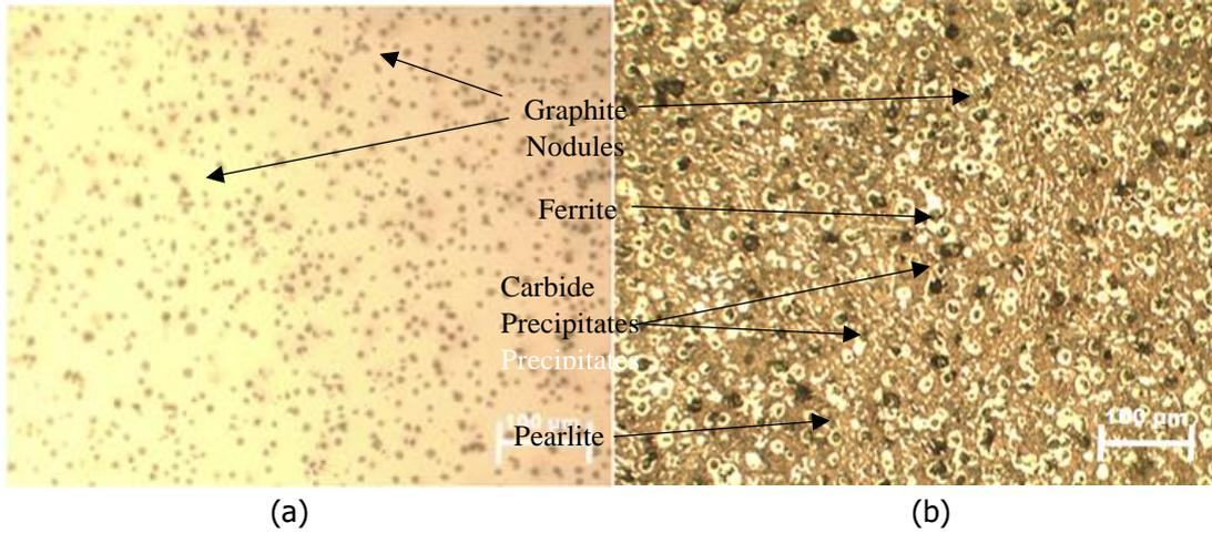
Figure 9: Micrographs of TWDI cast in Bentonite bonded sand (a) Unetched (b) Etched
