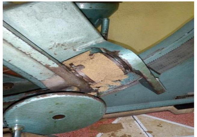
*Figure 3: Green Compression Testing using Ridsdale Sand Compression Tester*
