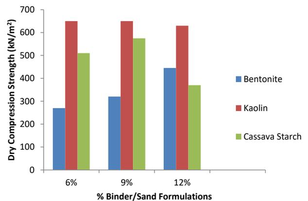
Figure 6: Dry Compression Strength with %binder/Sand Formulations
