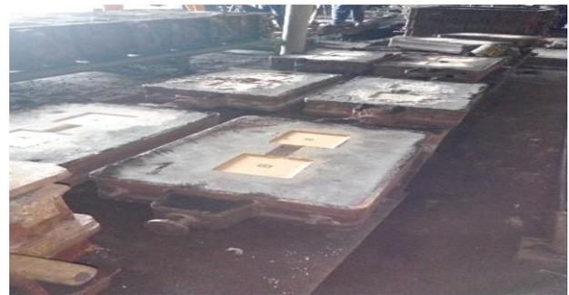
Figure 4: Cast TWDI samples in binder/ sand formulations
