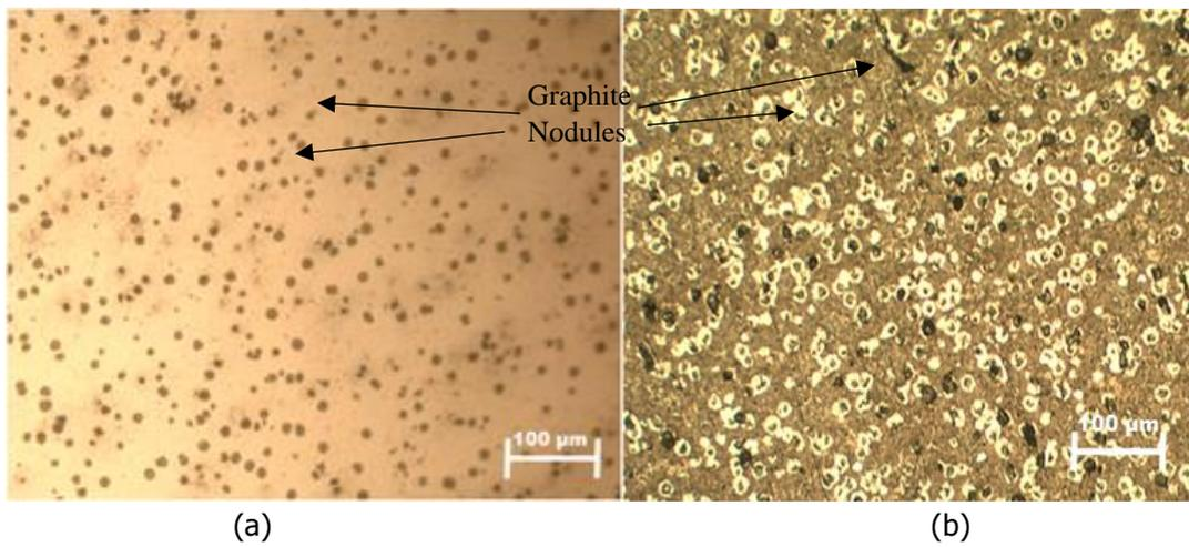
Figure 10: Micrographs of TWDI cast in Kaolin bonded sand (a) Unetched (b) Etched
