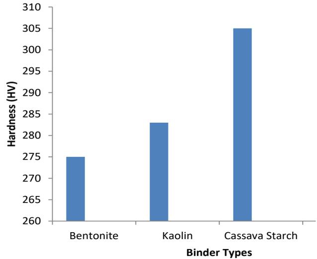
*Figure 8: Hardness of cast TWDI samples with Binder Types*
