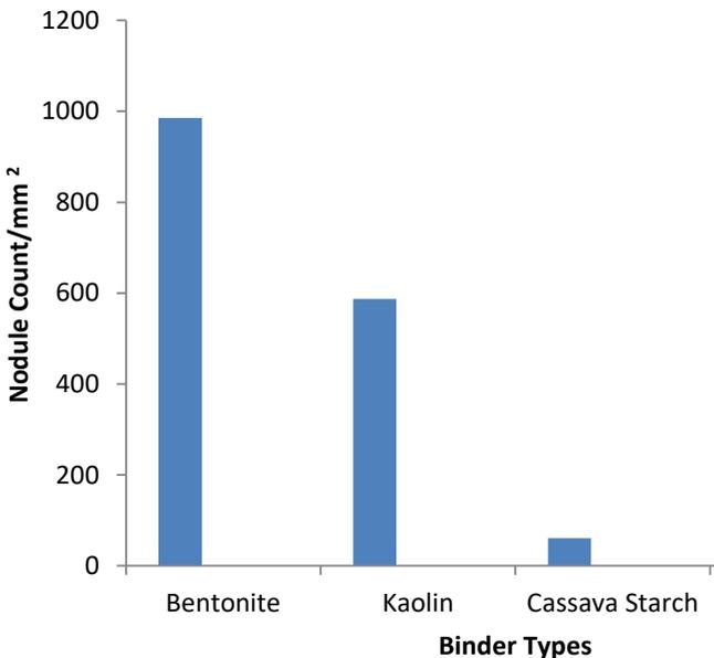
Figure 13: Nodule count/mm² of cast TWDI samples with Binder Types
