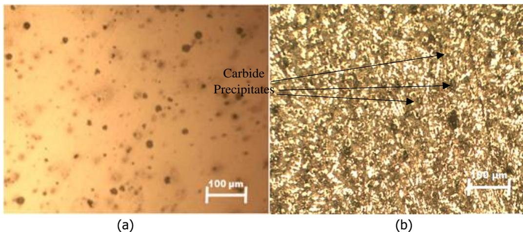
Figure 11: Micrographs of TWDI cast in Cassava Starch bonded sand (a) Unetched (b) Etched
