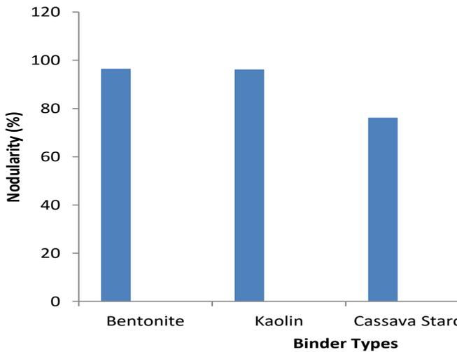
Figure 12: Nodularity (%) of cast TWDI samples with Binder Types
