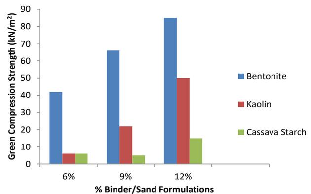
Figure 5: Green Compression Strength with %binder/Sand Formulations
