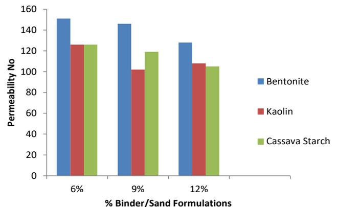
Figure 7: Permeability (No) with %binder/Sand Formulations
