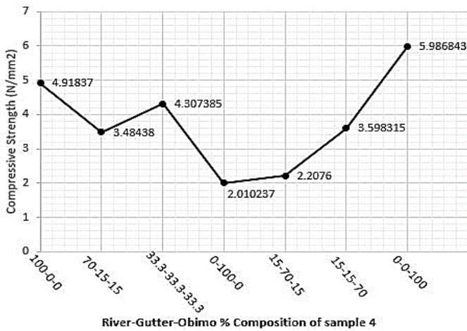
**Figure 4:** Compressive Strength of Sandcrete cubes at different percentages Composition of River-Gutter-Obimo sand
