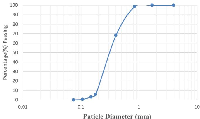
Figure 2: Particle size distribution of gutter sand
