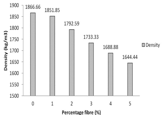
Figure 3: density of produced block samples
