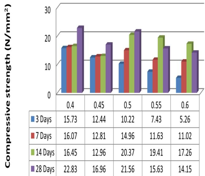
**Figure 4:** Compressive strength of sand-sawdust concrete versus water-cement ratio
