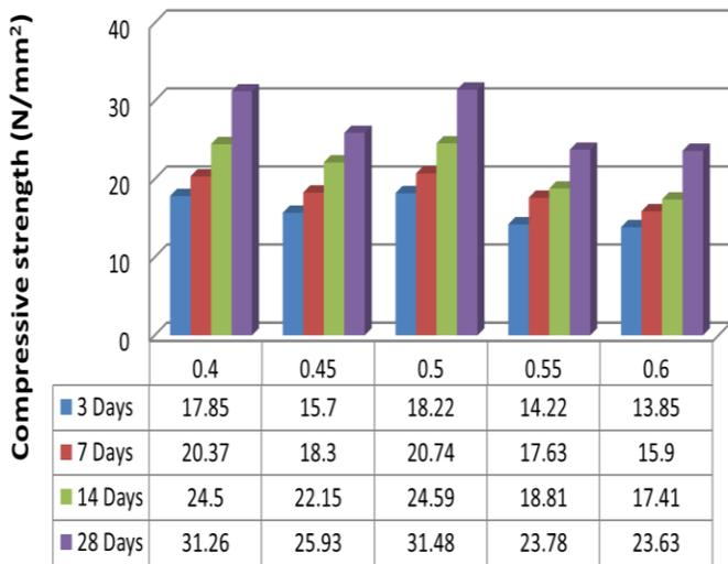
**Figure 3:** Compressive strength of standard concrete versus water-cement ratio
