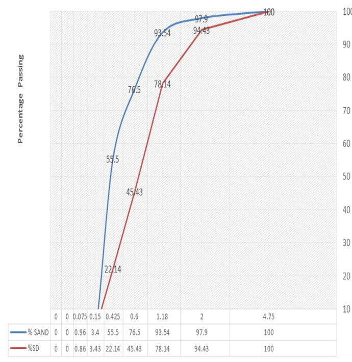
**Figure 1:** Grading Curves for Sand and Sawdust
