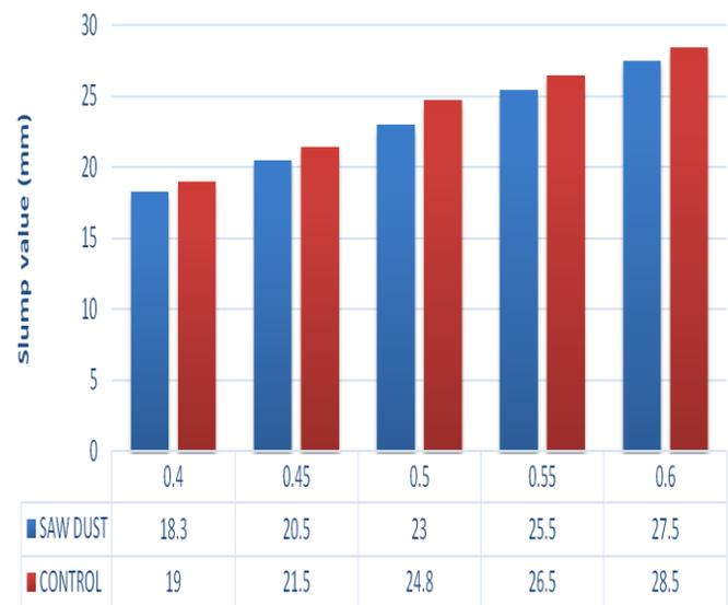
**Figure 2:** Comparative Variation of slump of concrete with water-cement ratio
