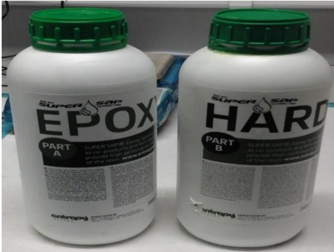
**Figure 1:** Super sap bio-derived epoxy and hardener used for the composite manufacture.
