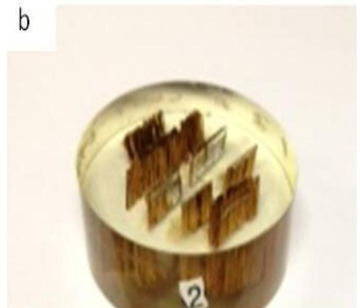
**Figure 7:** Potted, grinded and polished samples for optical microscopy (a) single coir fibre (b) coir fibre composites.
