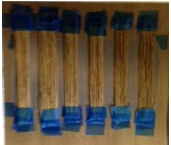
**Figure 3:** Coir fibre arrays in single layers
