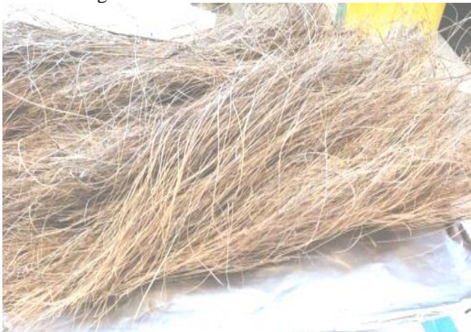
**Figure 2:** Washed and dried coir fibres
