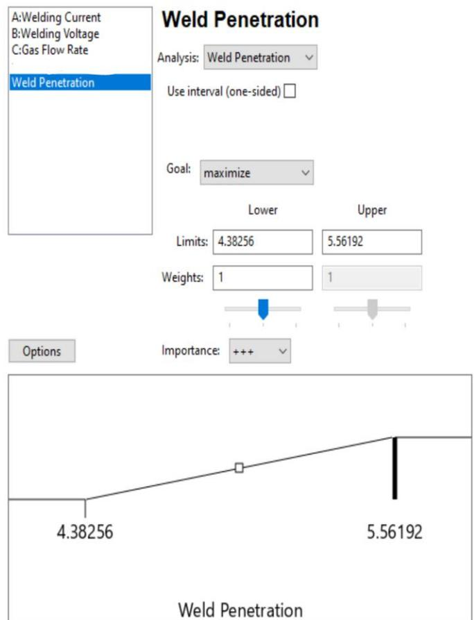
Figure 3: Interphase of numerical optimization of Penetration depth.
