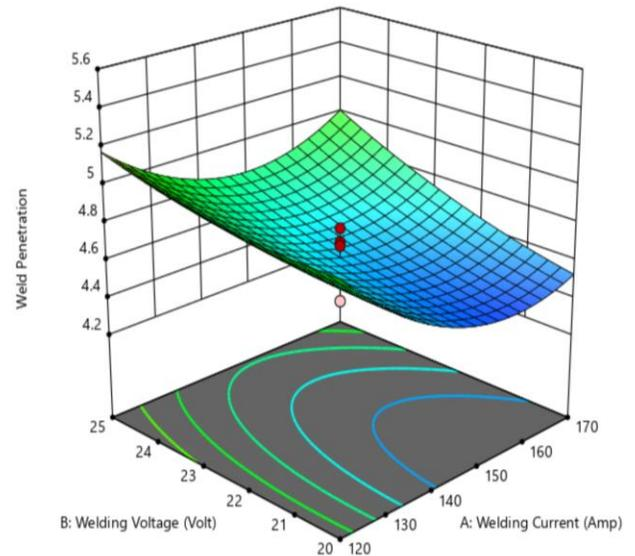
Figure 2: 3D surface plot for Penetration depth
