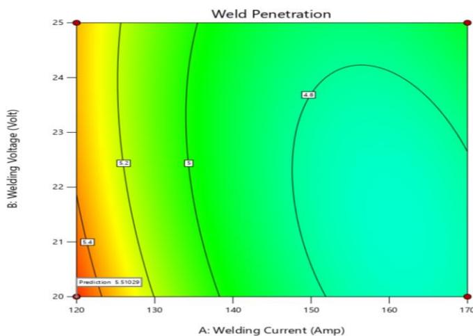
**Figure 4:** Predicting weld penetration depth using contour plot
