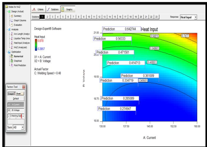
Figure 8: Predicting heat input using contour plot
