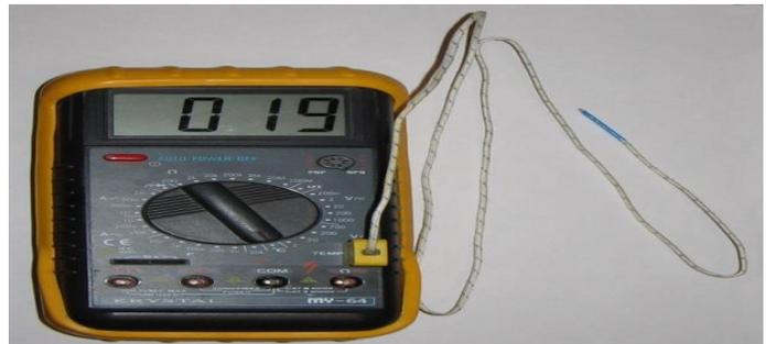
Figure 3: Digital thermometer
