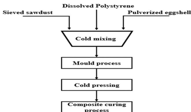
Figure 4: The processes of producing the composite samples
