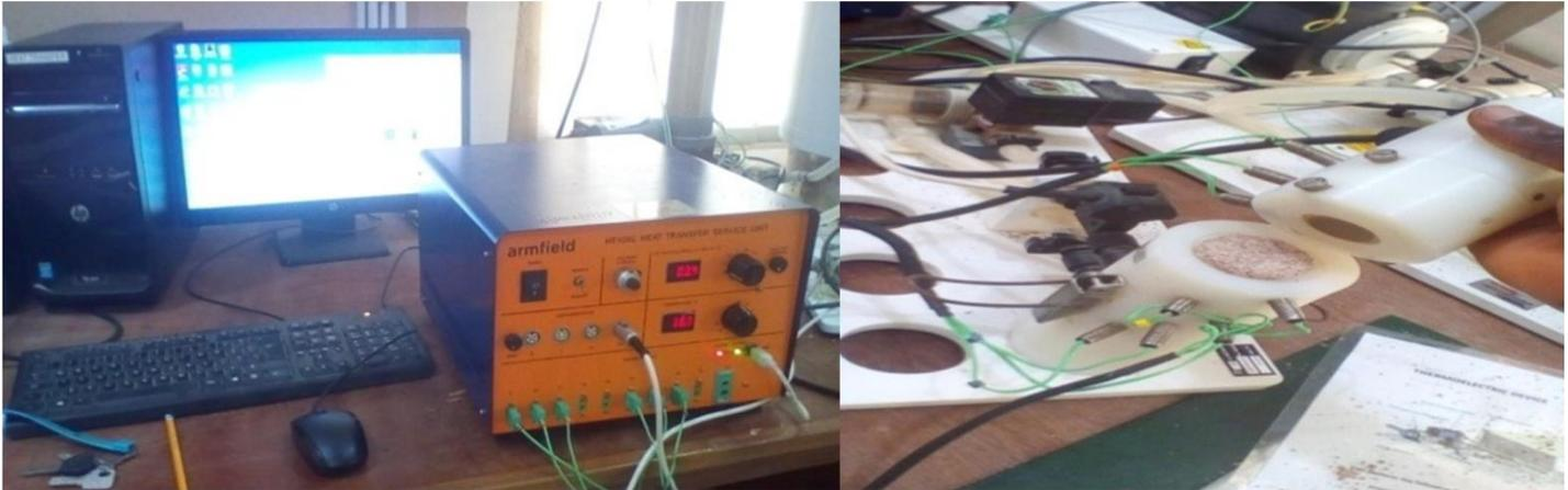
**Figure 6:** Computer compatible linear heat conduction apparatus setup for determining thermal conductivity.
