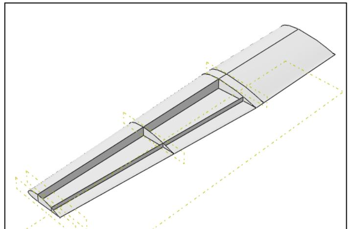
Figure 6: Model for final design FE Analysis
