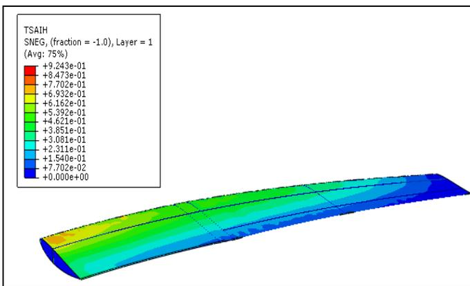
Figure 8: Tsai-Hill Failure Index- Max at 0.92
