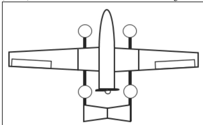
**Figure 1:** Hybrid UAV wing configuration
