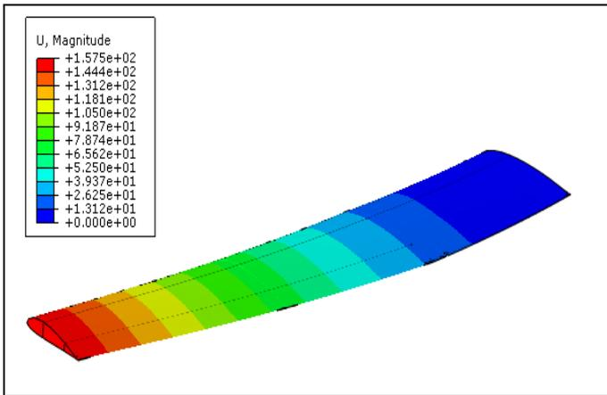
Figure 7: Magnitude of Wing Deflection -Max 157.5mm
