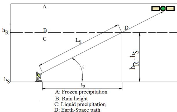
**Figure 1:** Slant Path through Rain [22]
