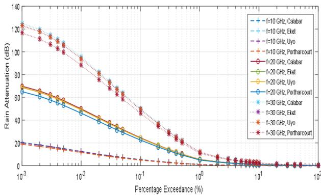
**Figure 6:** Variation of rain attenuation for Calabar, Eket, Uyo and Port-Harcourt at 10GHz, 20GHz and 30GHz.
