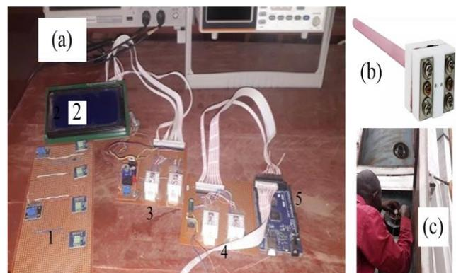
**Figure 2:** Experimental set-up: (a) Electronic Interface (b) Thermocouple Probe and (c) Thermocouple Probe Installation
