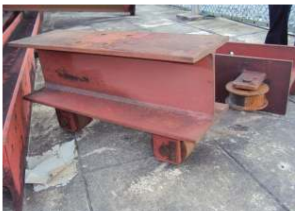
Figure 12: Part of clamp carriage showing rollers.
