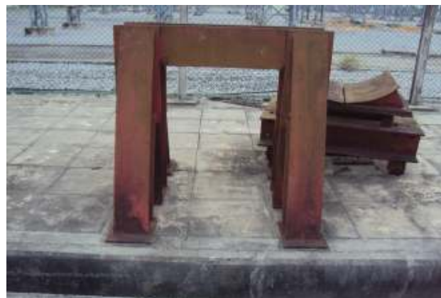
Figure 13: Pulling jack stand with saddle carriage.
