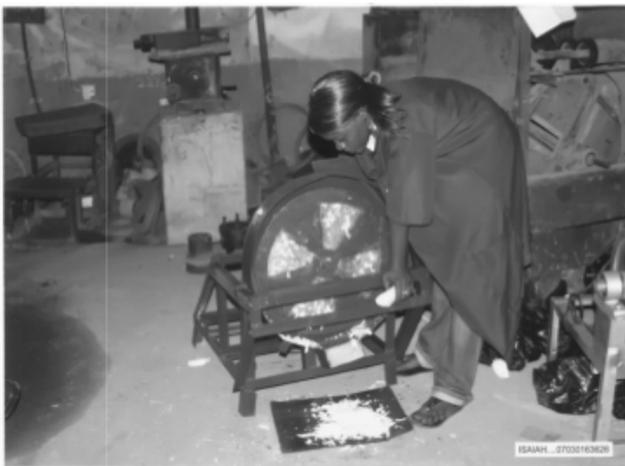
Figure 3: A student demonstrating the developed cassava shredding machine.
