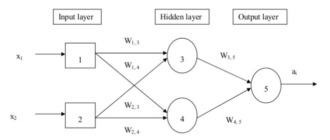
Figure 2: Two-input feed forward neural network model.
