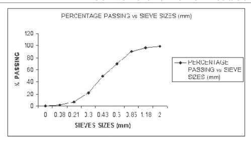
Figure 4: Grading curve for the fine aggregate.
