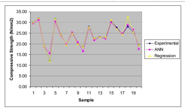
Figure 6: Comparison of ANN with experimental results and regression model prediction (granite).
