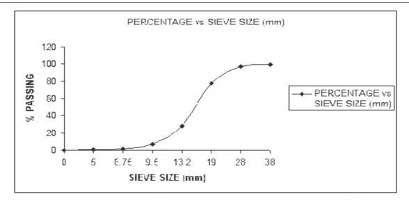
Figure 5: Grading curve for granite.
