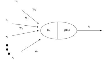
Figure 1: An artificial neuron. ( $W_i$  = weights;  $x_i$  = inputs;  $a_i$  = output)
