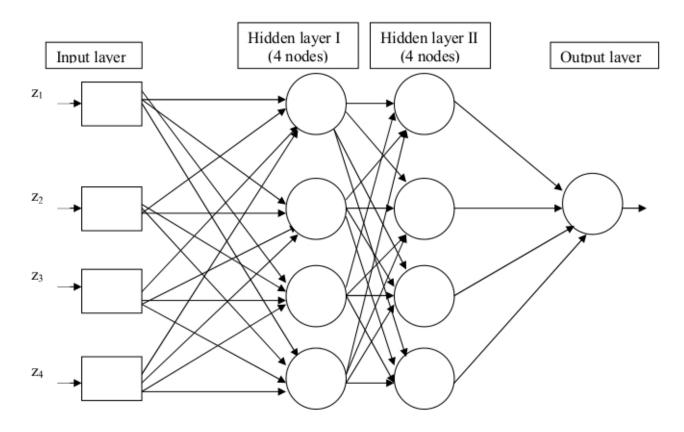
Figure 3: The Four-input, 4 layers feed foreword neural network model.
