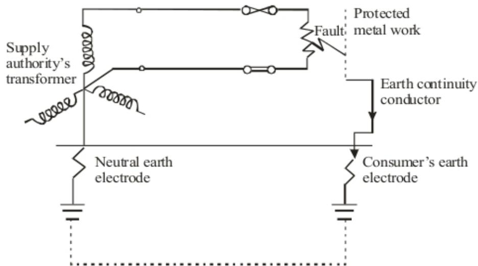
Figure 1: Earth fault loop-path.
