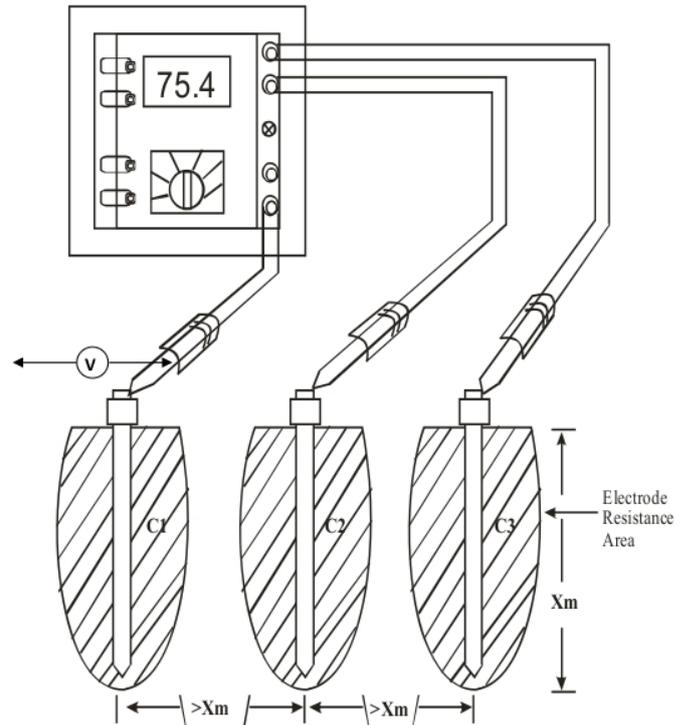
(a) Setup for testing soil resistivity using the fluke 1625
