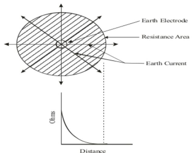
Figure 2: Earth electrode resistance area.
