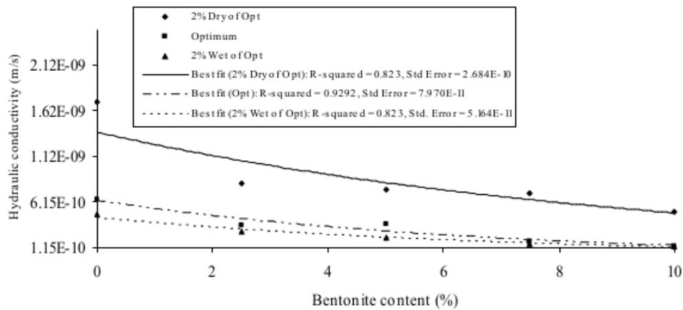
Figure 5: Variation of hydraulic conductivity with bentonite content.
