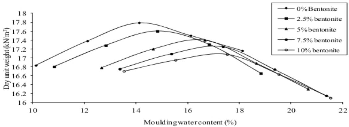
Figure 3: Compaction curves for soil mixtures containing 0, 2.5, 5, 7.5 and 10% bentonite.
