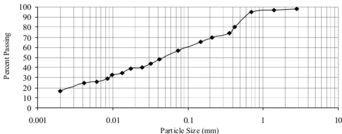
Figure 1: Particle Size Distribution Curve of Lateritic Soil.
