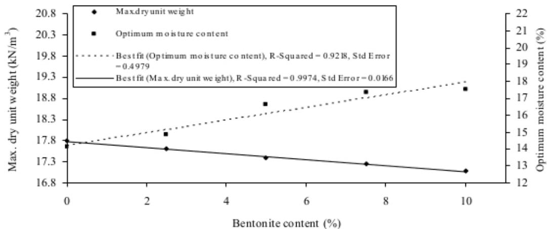
Figure 4: Variation of maximum dry unit weight and optimum moisture content with bentonite content.
