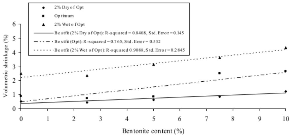
Figure 6: Variation of volumetric shrinkage strain with bentonite content.
