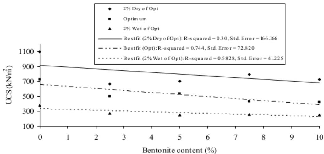
Figure 7: Variation of unconfined compressive strength with bentonite content.
