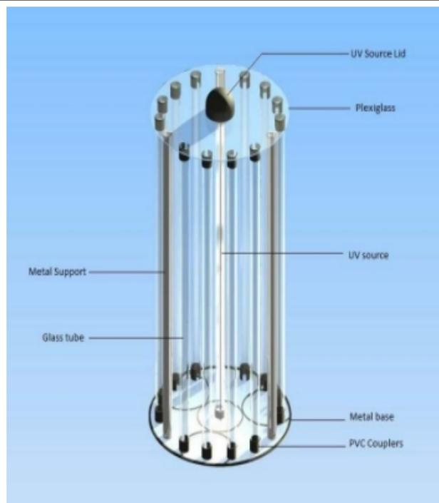
Figure 1: General arrangement of the photobioreactor.
