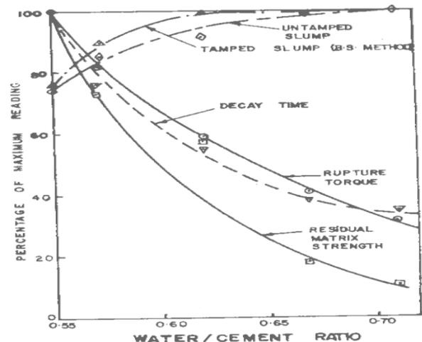
**FIG. 8. CORRELATION OF VARIOUS MIX PARAMETERS WITH WATER CEMENT RATIO.**
