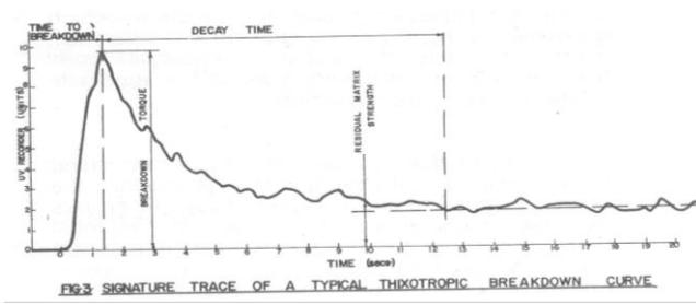
FIG.3 SIGNATURE TRACE OF A TYPICAL THIXOTROPIC BREAKDOWN CURVE.
