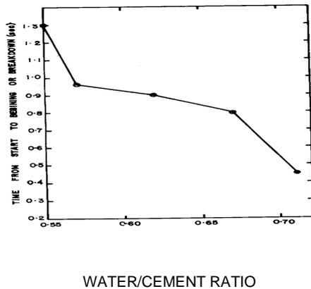
FIG-4. VARIATION OF TIME TO BREAK-DOWN WITH WATER/CEMENT RATIO (ROTOR SPEED 4 RPM)
