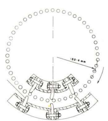
Fig.7. Section at the shelling unit showing the concave in two parts (cylinder rotates in the
