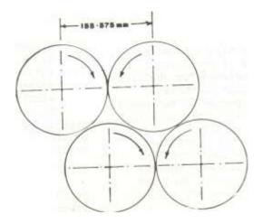
Fig.l. Schematic layout of the knurled roller machine
