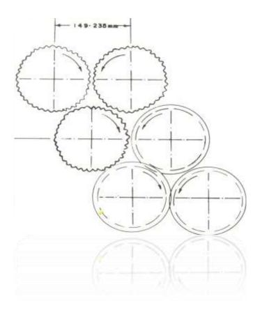
Fig.5. Schematic layout of machine showing the rollers with flutes parallel to the axis (top left) and rollers with flutes parallel to the circumference (bottom right)
