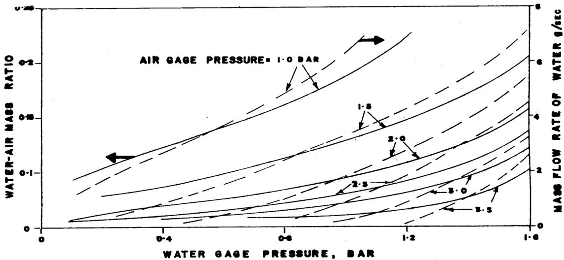
Fig. 1 spray Nozzle flow characteristics
