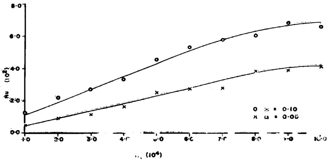
Fig. 7. Influence of stream velocity on rate of cooling
