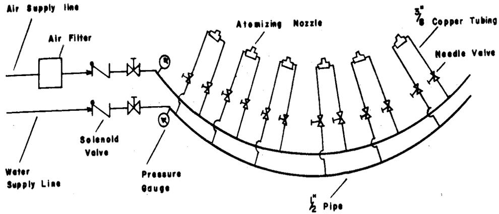
Fig.2 schematic diagram of the cooling unit
