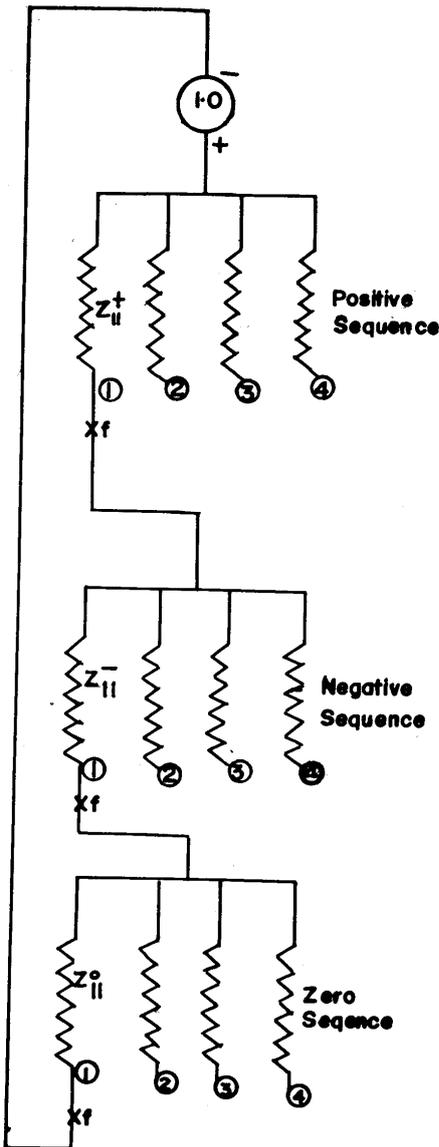
Fig. A1. Intersequence connection for S-L-G Fault.
