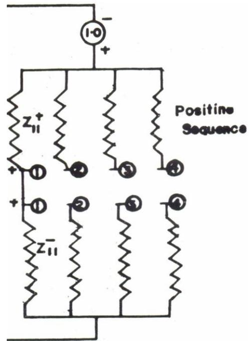
Fig. A2. Intersequence network for L-L fault at Bus 1
