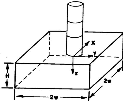
Fig.1. Basic configuration of a semiconductor device mounted on a finite heat sink.
