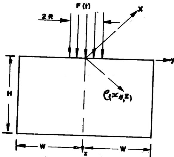
Fig.2. Side view of the heat source-heat sink geometry considered.
