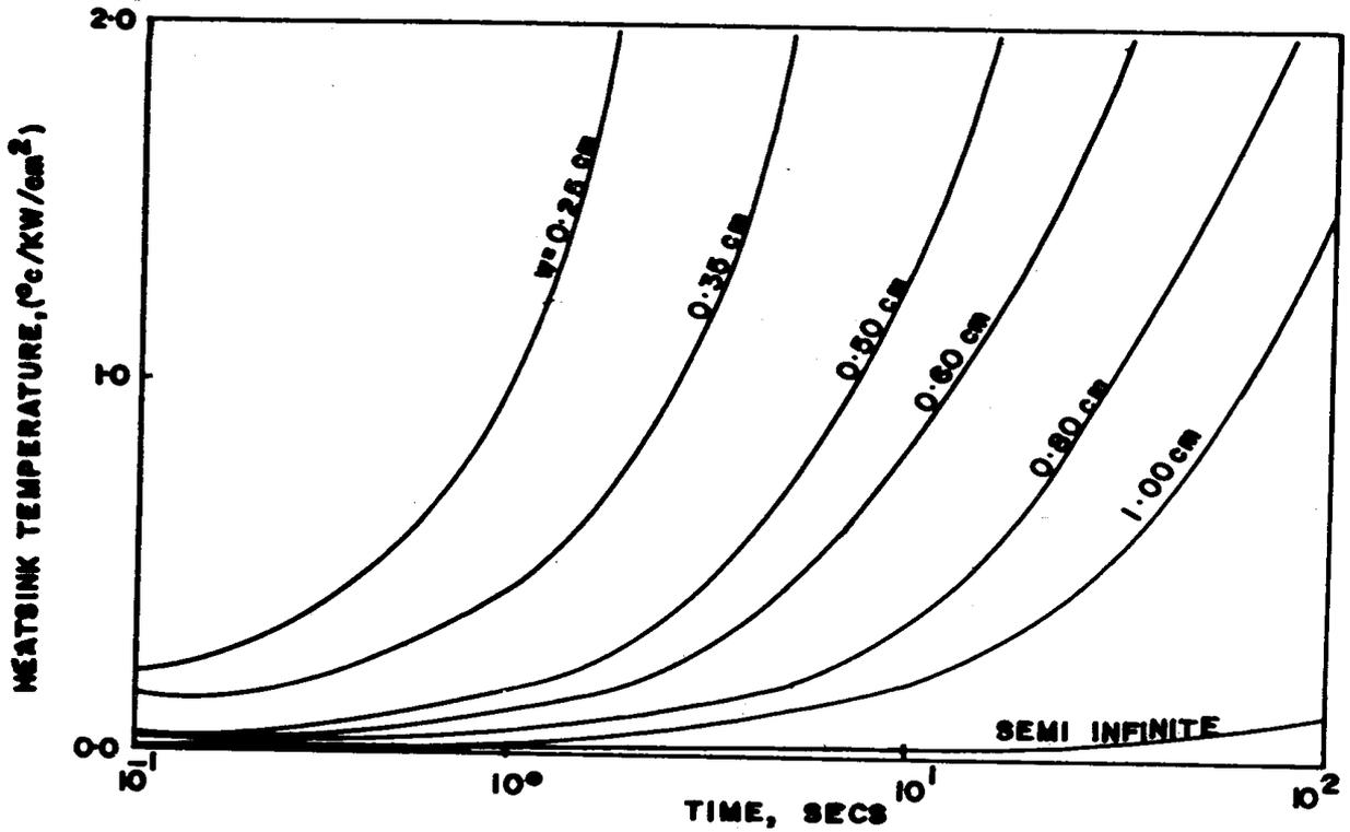
Fig.3. Heat sink temperature rise Vs time ( $H/W = 0.5, D = 1\%$ )
