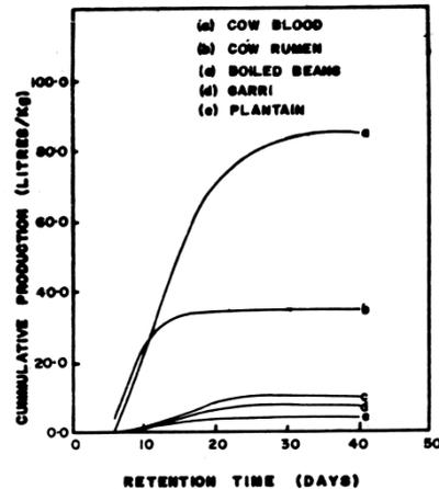
Fig. 2. Cumulative biogas yield from the various waste food materials.
