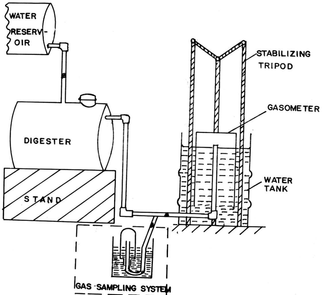
Fig. 1. Schematic of pilot plant.
