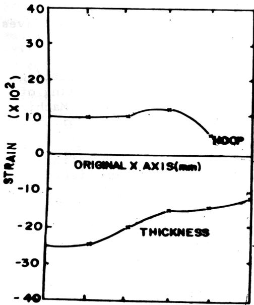
Fig. 8. Strain distribution for well-formed blanks.
