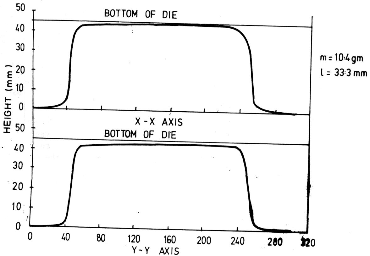
Fig. 6. Deformed blank profile in X -X and Y - Y direction for die base plate No. 2 of fig. 2.
