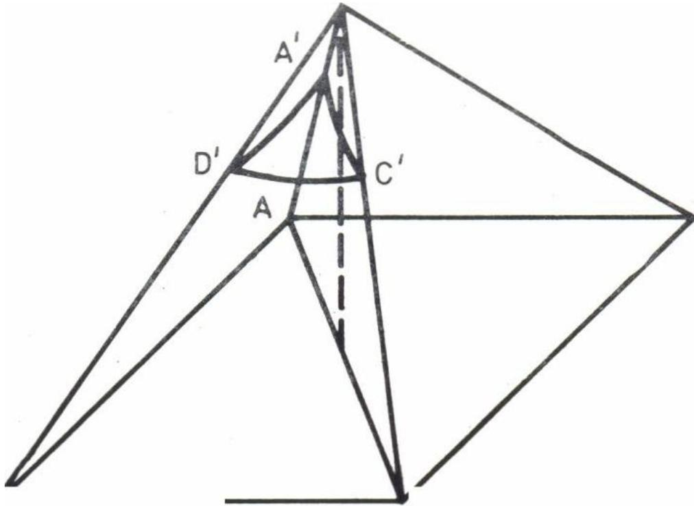
Fig. 1. Solid angle subtended by square blank ABCD at charge center O
