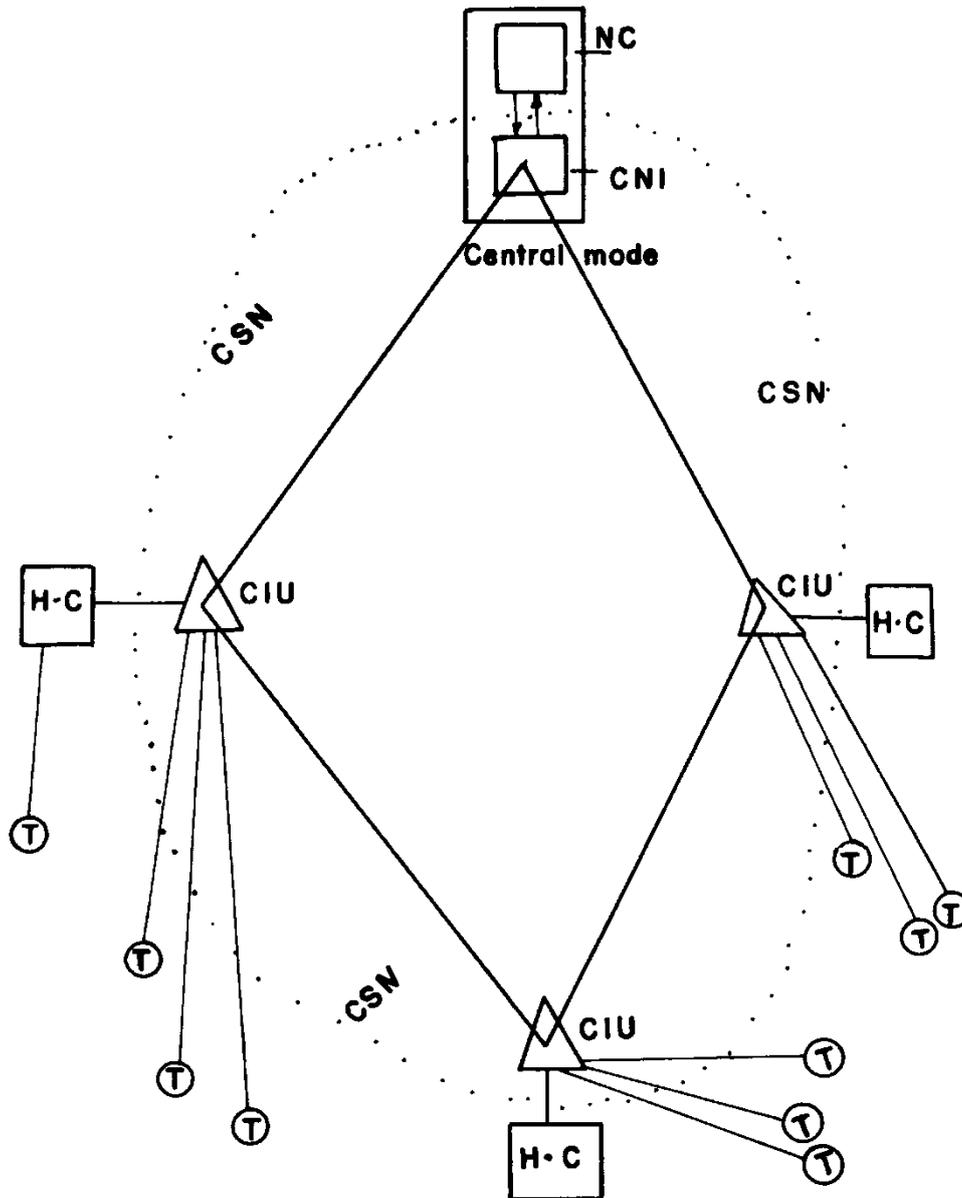
**Fig.1. centralized or star network**
