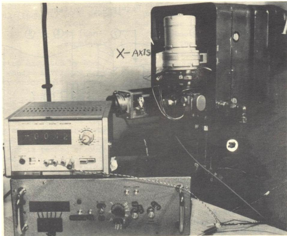
Fig. 1b: x-axis : main gearbox, new servo unity and control boxes.
